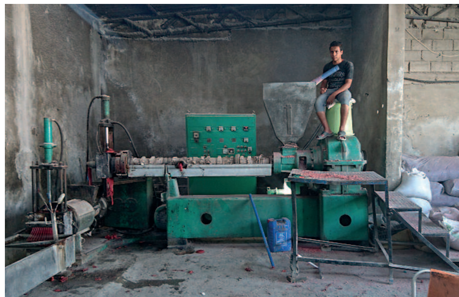
And reused: pellets being fed into the plastic recycler
